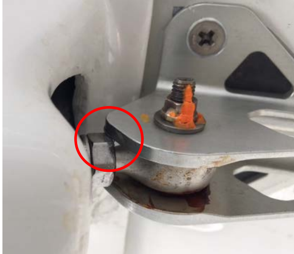
Figure 1: Interference between elevator control horn and elevator push rod jam nut
