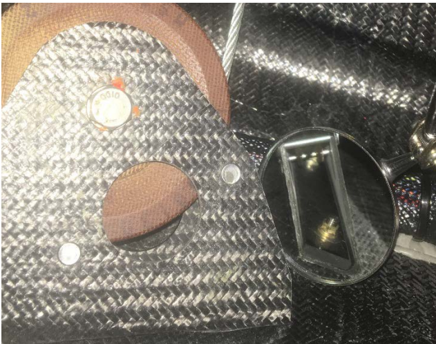
Figure 5: Roll Pulley Bracket Stud with carbon shim, washer and retaining nut. S/N 00013-current)
