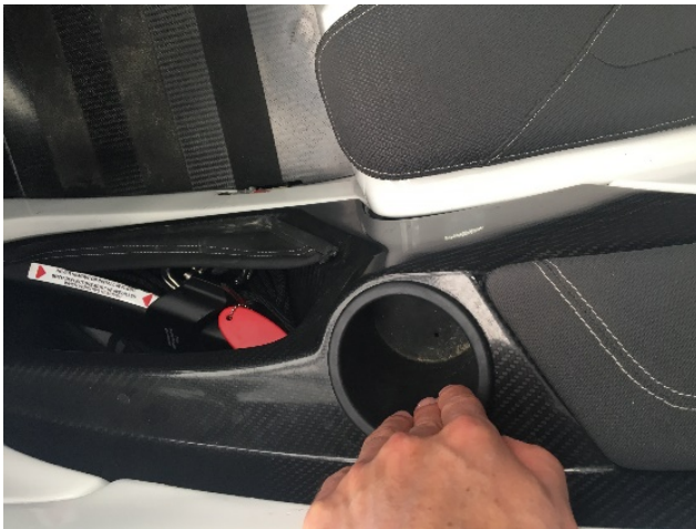
Figure 1: Compress cup holder walls, and lift cup holder out of the main cockpit side panel.
