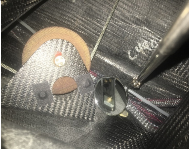
Figure 3: Roll Pulley Bracket Stud with aluminum shim block, and nut. (S/N 00001-00003)
