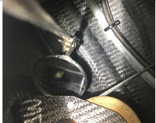
Figure 4: Roll Pulley Bracket Stud with nut and washers only. (S/N 00004-00012)
