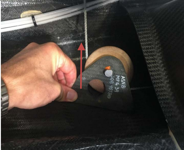
Figure 7: Pull on the bracket away from the fuselage skin wall once the cable is slacked to determine that studs clamp the bracket to the wall.
